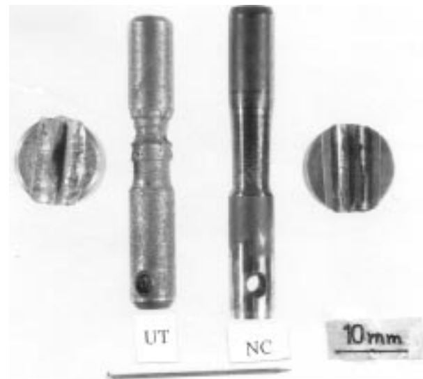
Fig. 6 Modes of failure in Falex test. UT, untreated; NC, nitrocarburized
